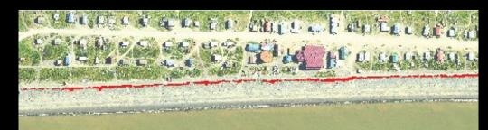
Erosion of berm fronting Shaktoolik (red) Area of erosion: 110,000 sq. ft Amount of erosion: 350,000 cubic ft
